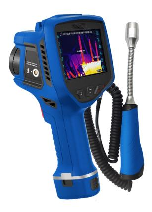
SATIR PD600 is a new release that is a thermal and partial discharge detector. This model offers both thermal imaging and a PD detector in one. It is ideal for the electrical engineers to detect potential issues within the sub stations and electrical applications
