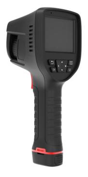
SATIR are pleased to announce the release of the i-384 New, an industrial handheld thermal camera series. the i-384 New which is a mid-level thermal camera as it has 384x288 IR resolution.
