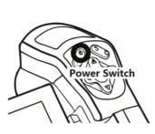
Press and hold the power switch for 3 seconds. The power indicatior lights green.
